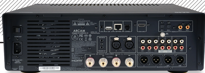
ABOVE: MM/MC, four line inputs (one balanced on XLR) are joined by two preamp and filtered sub outputs (RCA and XLR), with digital on two optical, two coaxial, USB-A and HDMI eARC. Bluetooth 5.4 is supported alongside Wi-Fi and wired Ethernet (up to 384kHz/32-bit), and note the pairs of chunky 4mm speaker sockets
