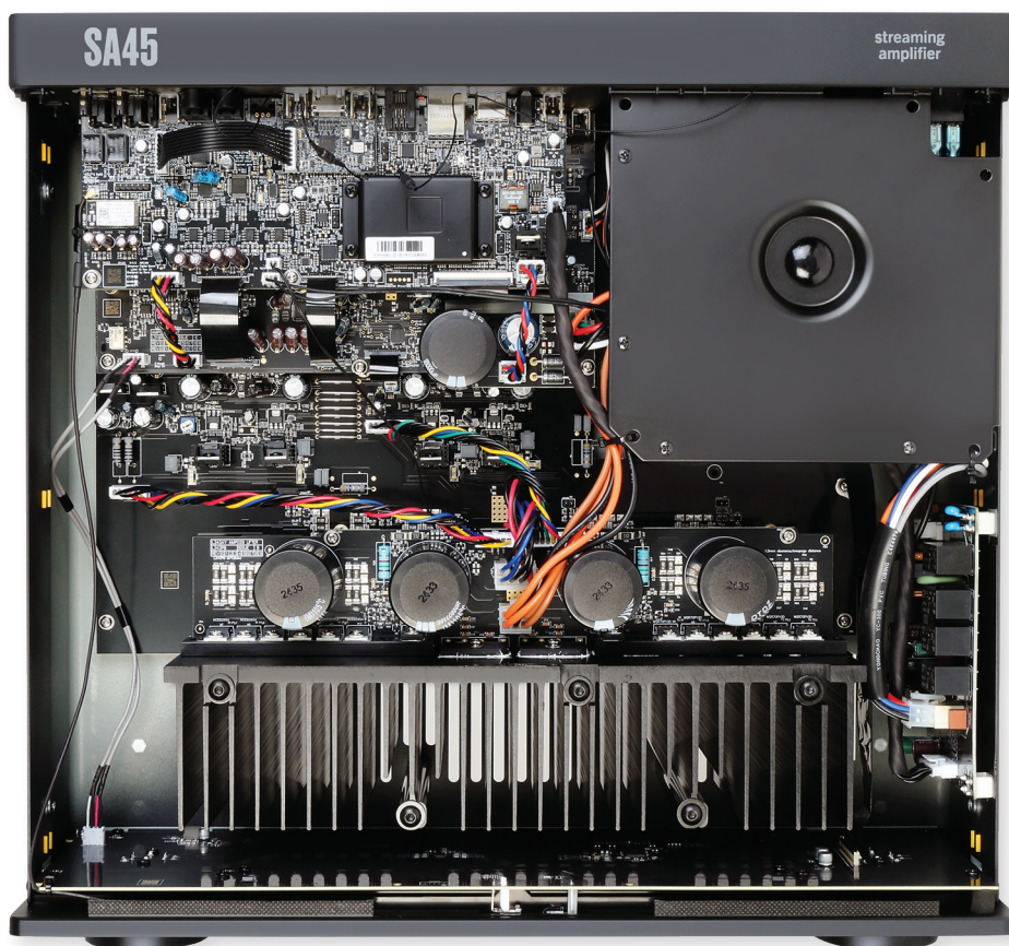
RIGHT: Massive toroidal transformer [top right] services the Class G PSU/amp [bottom]. Multi-layer PCBs [top left] host network module, HDMI eARC input, ES9027S Pro DAC, MM/MC phono stage, line in and isolated preamp outputs
