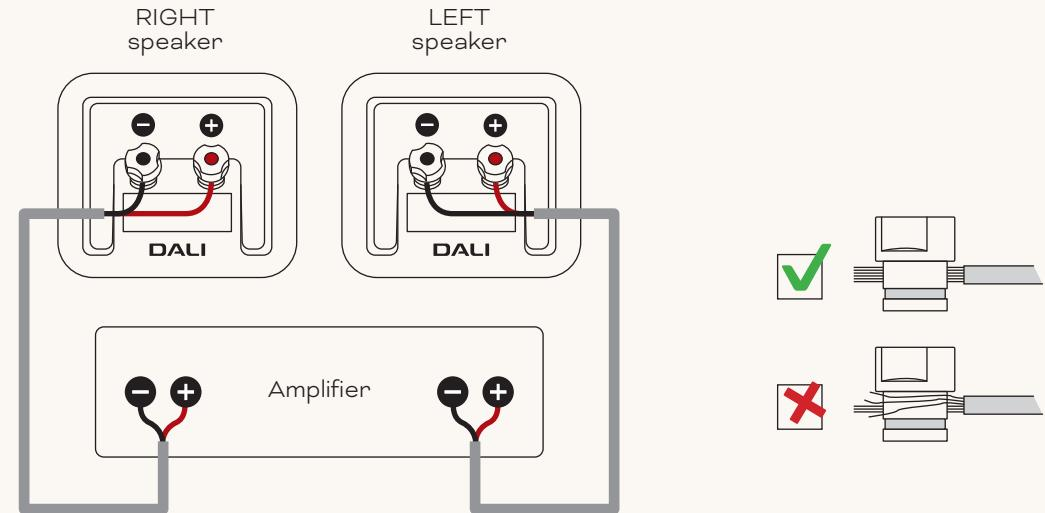
! Make sure that the bare conductors are tightly gripped by the terminals with no loose wires which could cause a short circuit and damage the amplifier.
