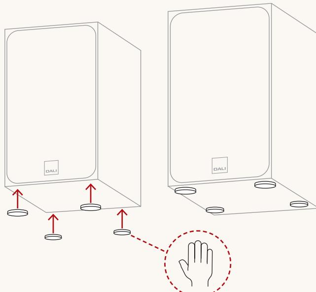
If hanging SONIK 1 on a wall, mount the rubber feet on the rear edges of the loudspeakers. To hang the loudspeaker on a wall, use one screw mounted in the wall. The screw must fit the wall bracket on the rear side of the loudspeaker.
