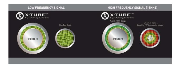
At low frequencies both X-Tube™ and conventional stranded/solid core speaker cables convey signals in a linear way. However, at high frequencies, X-Tube™ retains a near-linear signal transfer, whereas the conventional cables fail to conduct uniformly across the entire conductor area.
